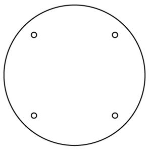
2. Drill four holes according to the supplied **Template Plate**, and insert the supplied **Plastic Anchors** into the holes.
