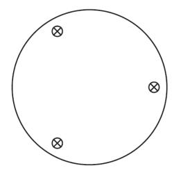
2. Drill three holes according to the supplied **Template Plate**, and insert the supplied **Plastic Anchors** into the holes.
