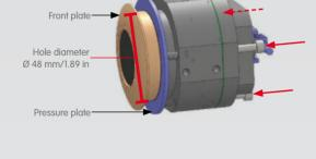
Tighten the cylinder head screws (red arrows) to push the pressure plate against the wall/faceplate Hole diameter Ø 48 mm/1.89 in Possible thickness of wall/faceplate: 0 to 14 mm/0 to 0.6 in
