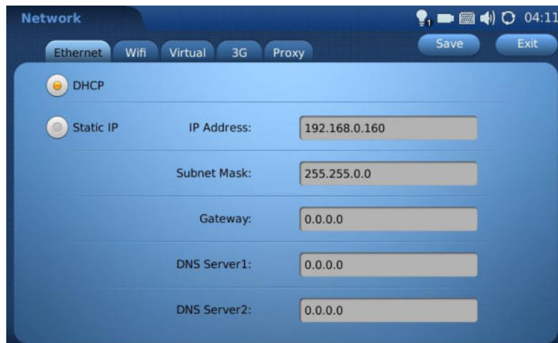
Figure 106: Network Settings → Ethernet
